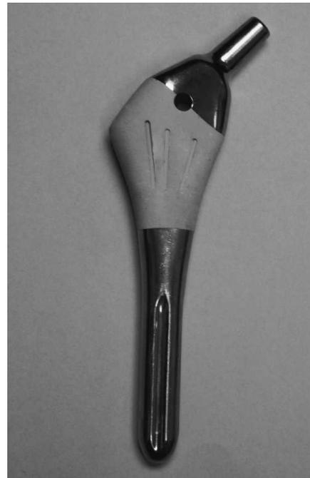
**Fig 1.** The custom-manufactured titanium lateral flare femoral stem is shown; the proximal 1/3 has a circumferential grit-blasted HA-coated surface. The prominent lateral expansion captures the lateral cortex. The distal stem is polished and has macrogrooves to limit bone contact.
