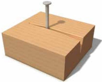
Fig. 1 - Initial Non-cemented Fixation. The analogy of non-cemented initial fixation to that of a nail in a piece of wood.
